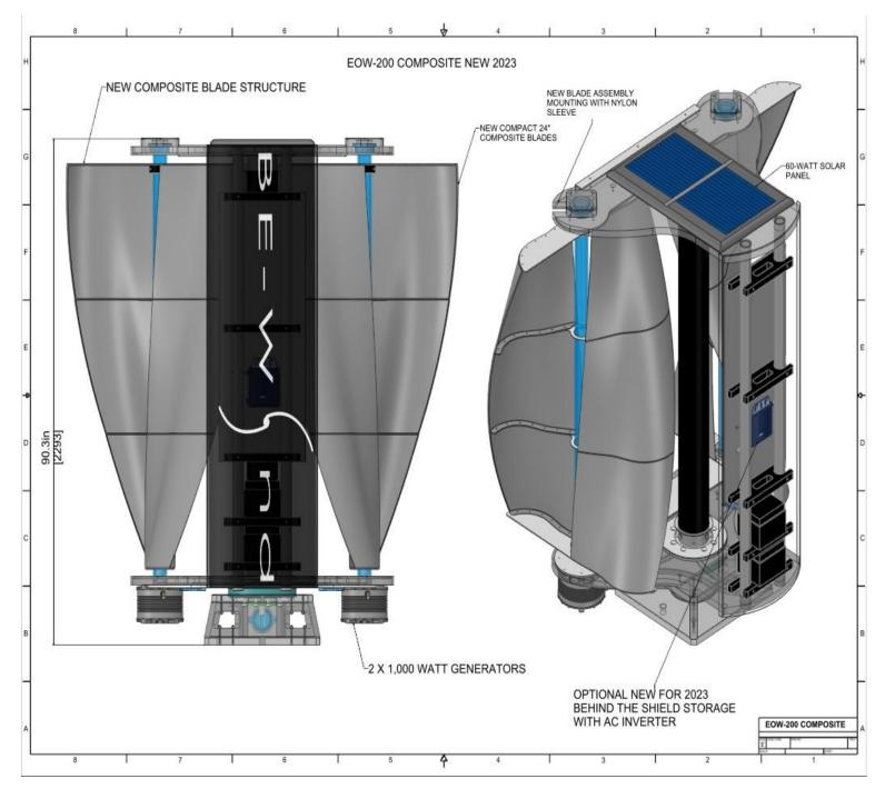
The EOW-200 series turbine is the flagship design by BE-WIND. Manufactured with HDPE ST structural marine grade plastic for the main Base and Top structures, The mounting and slew bearing attachment known as the universal base assembly.
